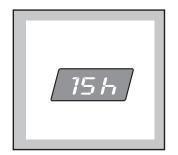
The delay time is displayed for 3 seconds, then the duration of the selected programme reappears. After you have pressed the "**Start/Pause**" button, the countdown begins, and the delay time value decreases by one unit every hour and then, when 2 hours remain, the time decreases in 30 minute intervals. You can delay the start of the selected programme by up to 23 hours in one hour intervals.
